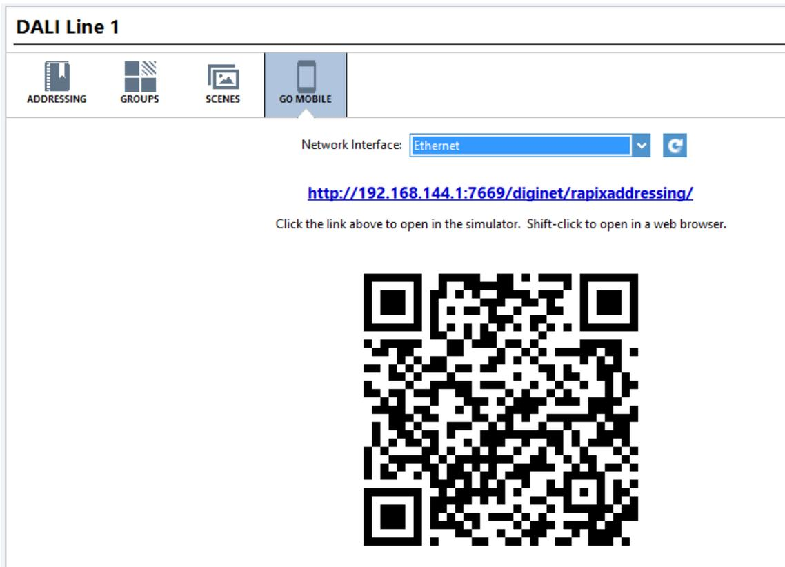
The Connect to Mobile Device window with combo box for choosing a network interface
