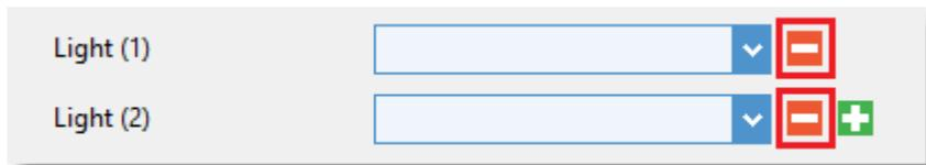
Two fieldbus addresses ready to be configured with the remove buttons highlighted
