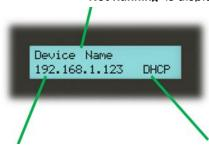
The Zone Controller IP Address is displayed here (or other information set by RAPIX Integrator software) DHCP is displayed if it was used to set the IP Address. If a static IP Address is used, then nothing is displayed here.
