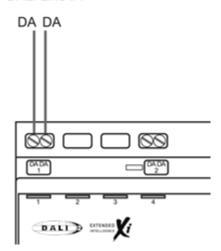
Up to two or four DALI lines (depending on model) can be connected to a Zone Controller. Each DALI line has two conductors which are not polarity sensitive. DALI line cabling must be double-insulated and mains rated.
