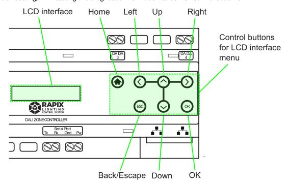
Figure 4 – Zone Controller User Interface
