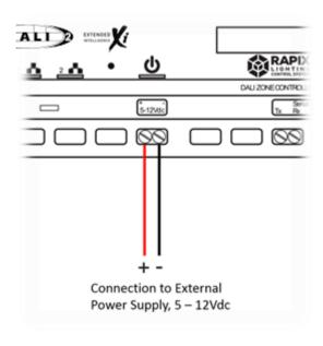
The Zone Controller is externally powered from a 5-12 V dc SELV power supply capable of supplying at least 200 mA @ 12 V dc (500 mA @ 5 V dc).
