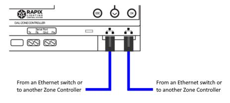
Ethernet is connected to the Zone Controller with standard Cat5e / Cat5 / Cat6 cable, terminated with RJ45 connectors.
