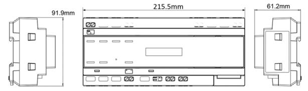
Figure 6 – Zone Controller dimensions
