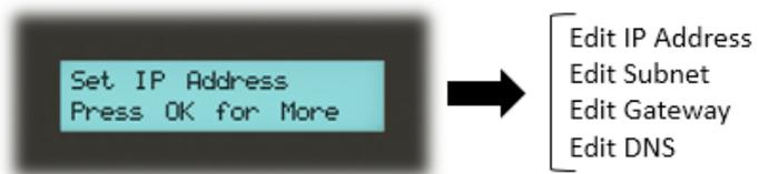
Note: The Zone Controller is set to DHCP mode by default. The unit can be changed from DHPC to Static IP Address mode via the 'Networking' menu (see next page).
